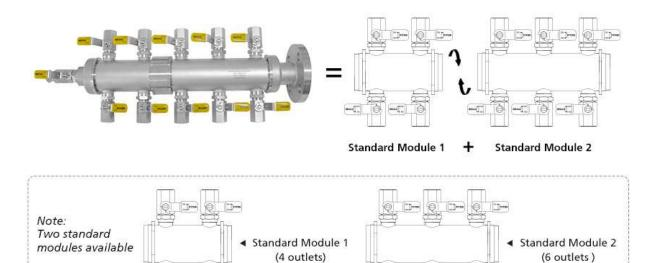
With modular design, an individual air header can be made up by several standard modules as shown above. FITOK air headers are available for sale as a complete set, or customers can order **4-outlet or 6-outlet standard modules** separately. This not only makes in-line upgrade and maintenance possible, but also save time and cost significantly. Every air header is **leak tested at factory with air or Nitrogen at rated working pressure.**
