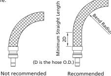
Maintain the minimum straight length for bent section, otherwise, hose rupture or leakage may result from bending too close to the hose/fitting connection.
