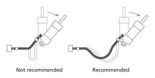
Elbow-connected hoses are better suited for vertical movement than hoses connected with straight fittings.
